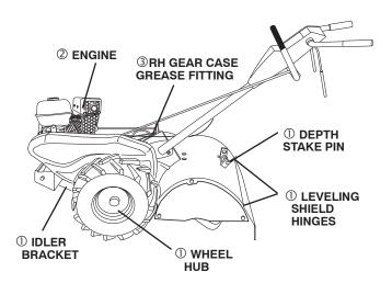
①SAE 30 OR 10W-30 MOTOR OIL ②REFER TO MAINTENANCE "ENGINE" SECTION ③EP #1 GREASE
